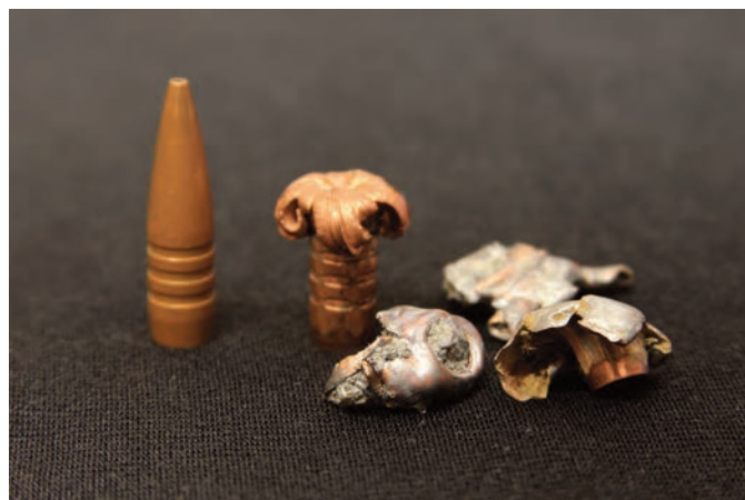
Copper ammunition (left) does not fragment like lead-based ammunition.
